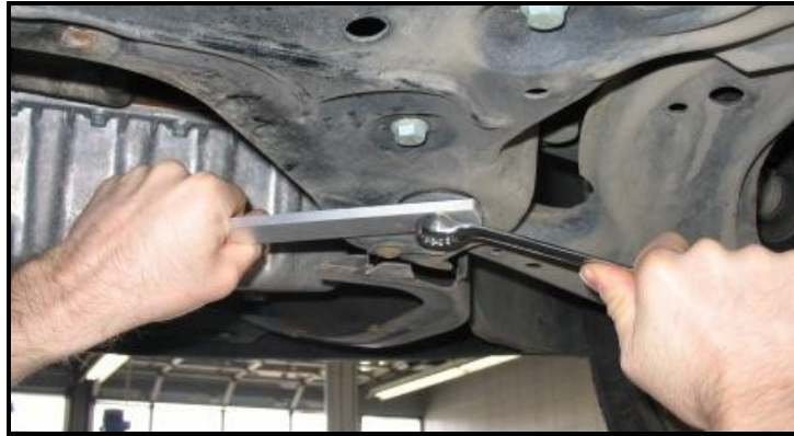
Picture F: How to install the Rivet Nuts on the rear sub frame.
