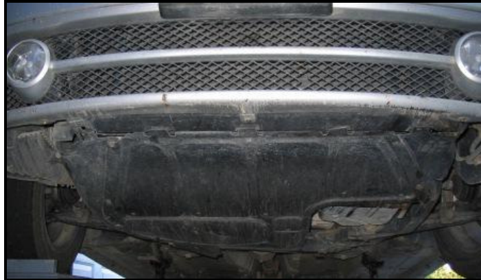
Picture A: Showing a plastic skid plate (TDI diesel).
