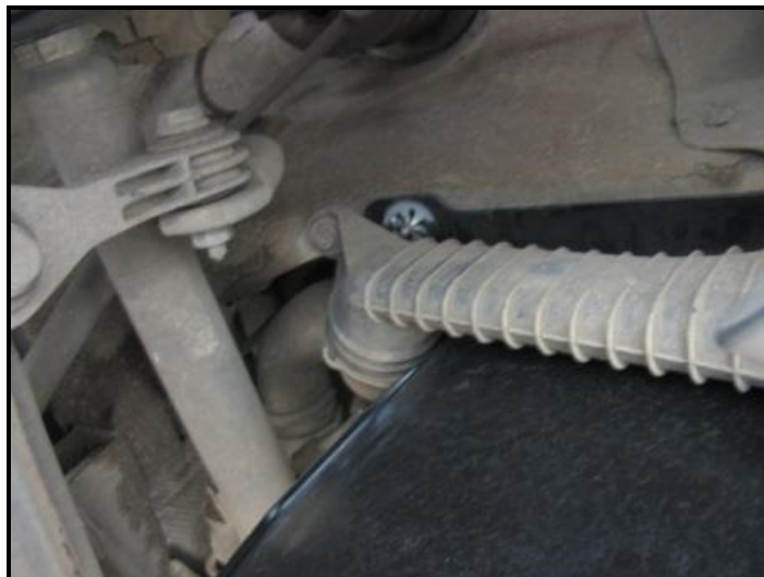
Picture B: Showing the round metal star clips on your side skirts. You will need to thread these off of the stationary bolts (two each side).
